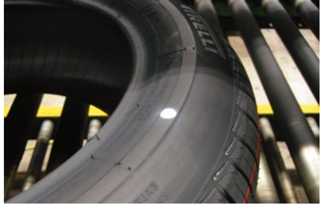
High-point marking on tires
