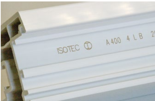
Coding and marking of plastic profiles
