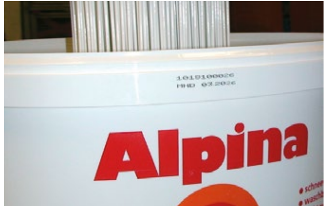
Marking of plastic paint buckets
