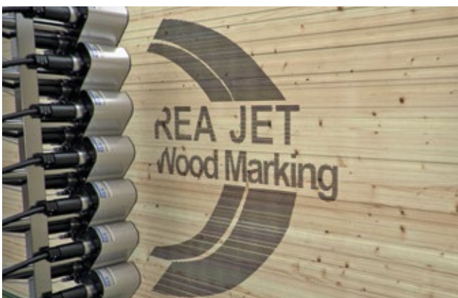
Large marking of logos on stacked boards
