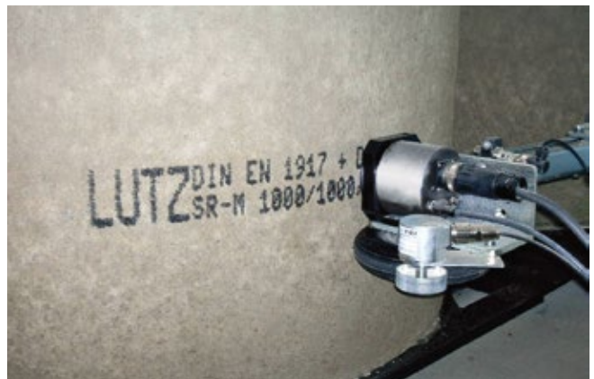
Marking of concrete pipes
