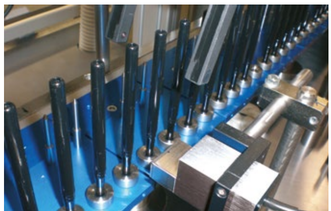
Precise application of oil on plastic parts
