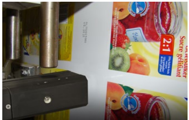
Marking of packaging foils
