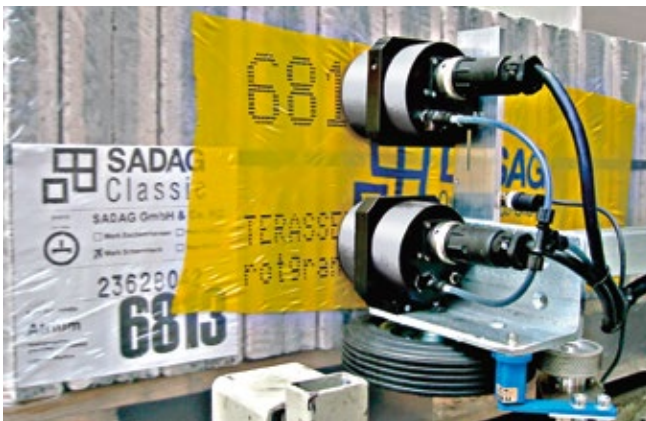
Coding and marking of shrink hoods
