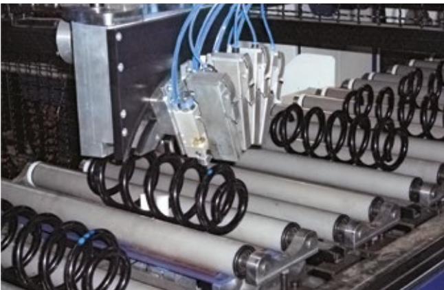
Marking of steel springs for type classification
