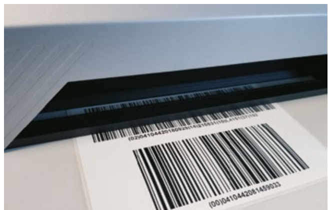
Quality verification of barcodes
