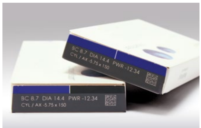
Coding and marking of packaging through color removal
