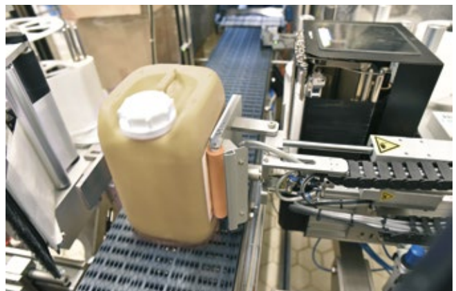
Multi-sided canister labeling
