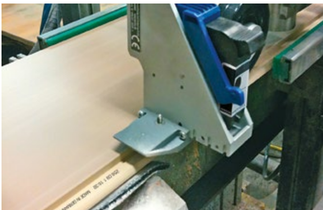
Coding and marking of laminate
