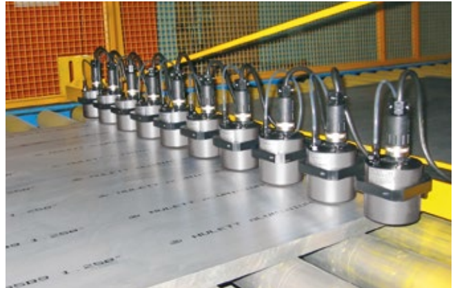
Marking of aluminum plates
