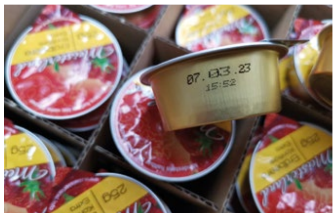
Best before date marking on jam tins
