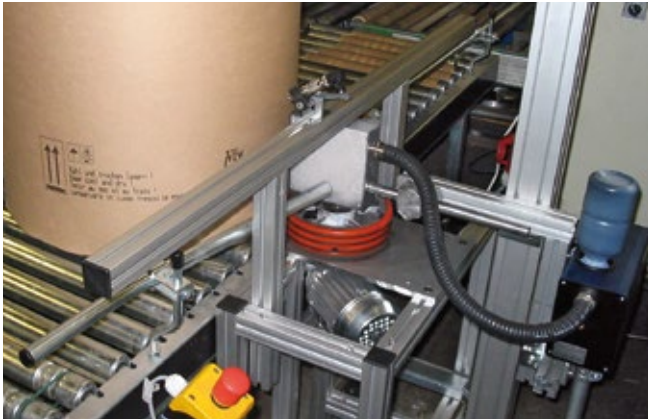
Coding and marking of fiber drums
