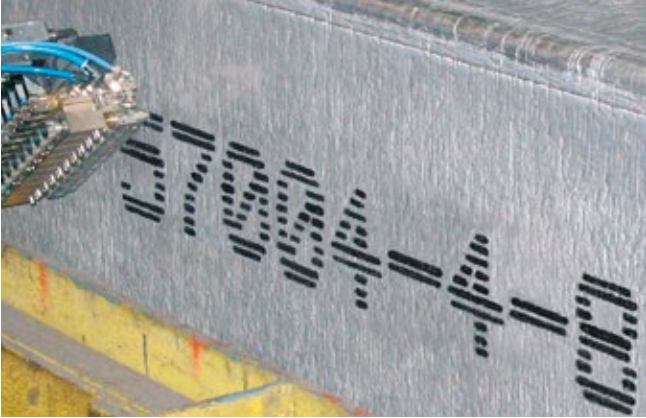
Marking of aluminum ingots
