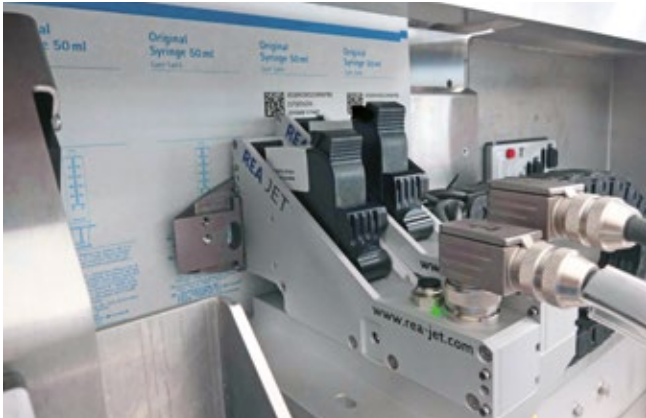
UDI marking of packaging material
