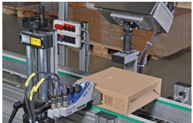
Marking cardboard boxes with barcodes
