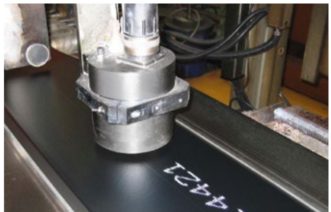
Marking of tread on raw rubber
