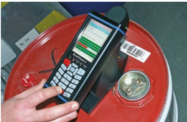
Verification of barcodes on metal drums
