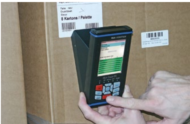
Flexible verification of barcodes on site
