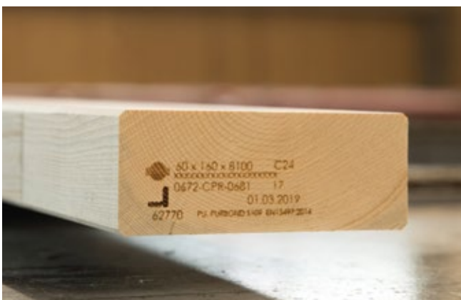
Wood marking with CO 2 laser
