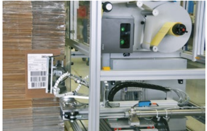
Pallet labeling (one stop for two sides)
