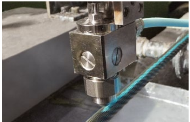
Color marking of wire cables
